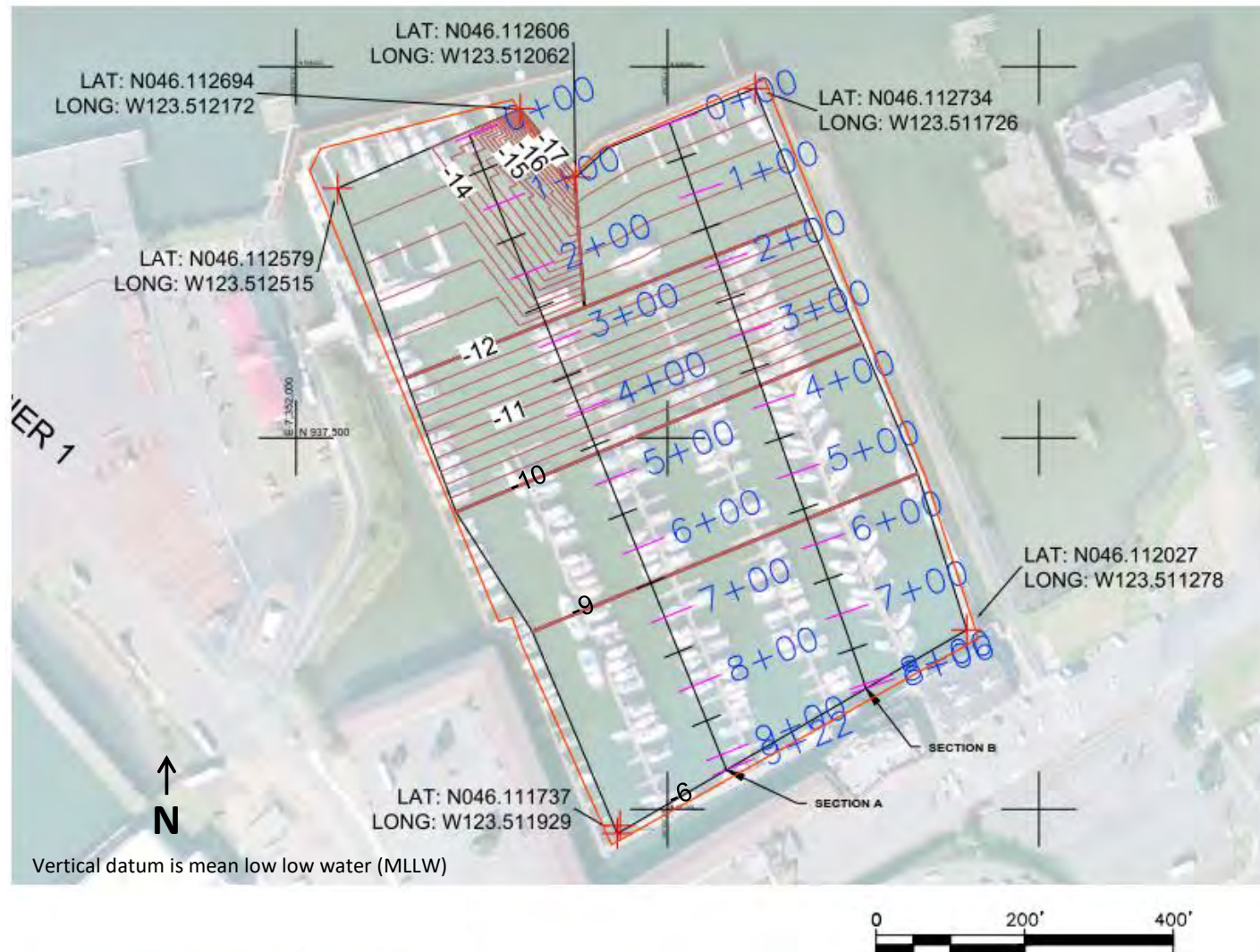
Figure 4B: Dredging Plan (Post-Dredging Surface)
