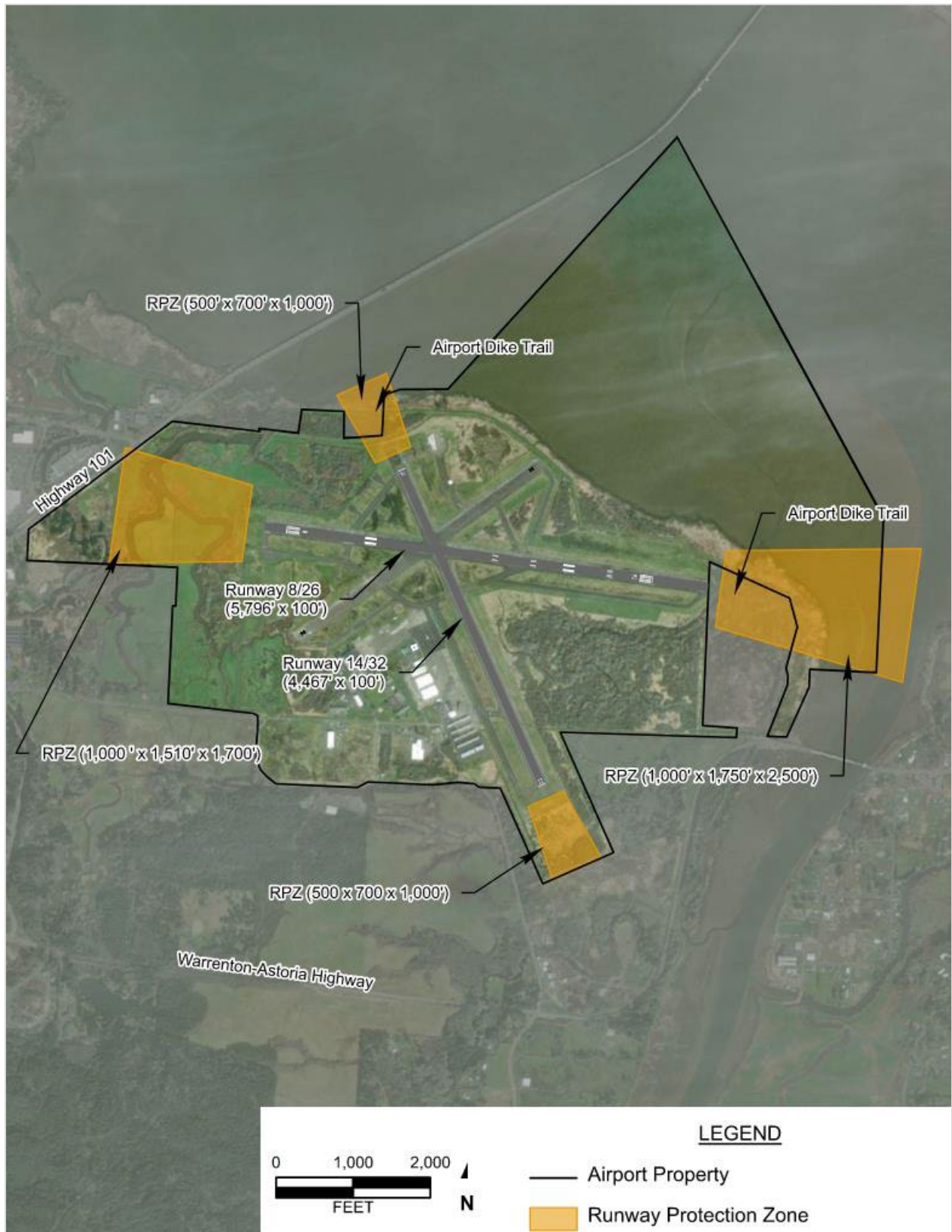
Figure 4-1: Runway Protection Zones
